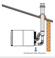
Balanced flue roof outlet (type C32)
